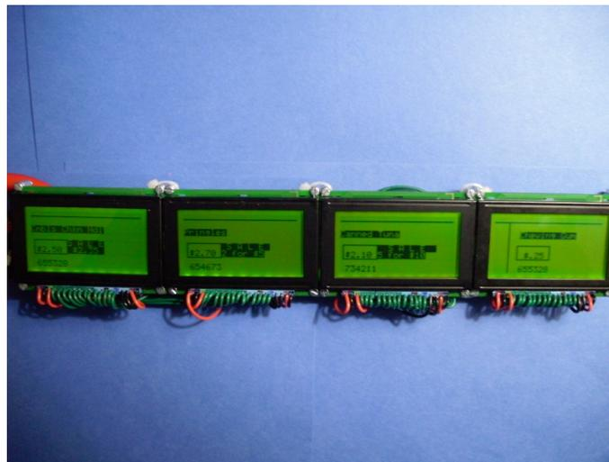
Figure 1: Digital Ad-Tag Display Modules
