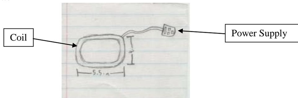
**Figure 9 - Flexible Double Coil**
