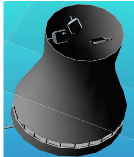
Figure 2: Cooling Tower Shell
