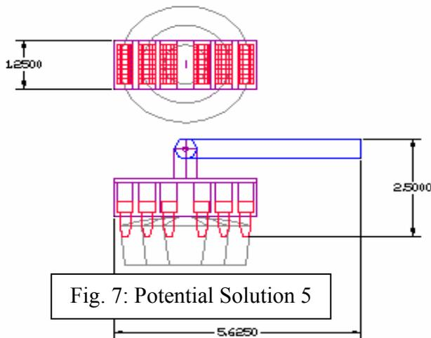
Gator Grip”. The pins that are in contact with the knob depress, leaving those in contact with the outside surface extended. The extended pins are in contact with the contours of the knob, thus creating a potential for turning force to be
