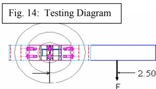
from the pivot point of the handle and force will be applied to the knob. The amount of force that can be applied in a horizontal direction
