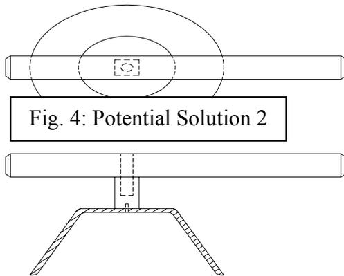
and a long handle to turn it with. This is the simplest solution. The conical section would have to have a contour on the inside of the conical section to afford it the proper amount of grip to turn the knob. This solution would require force to keep it from coming off of the knob, however it does
