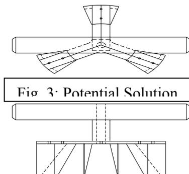
The first possible solution is based on an antique jar opener. The opener is designed so that as the handle is rotated the jaws on the ends close and apply the necessary force to grip the jar lid and allow the lid to be
