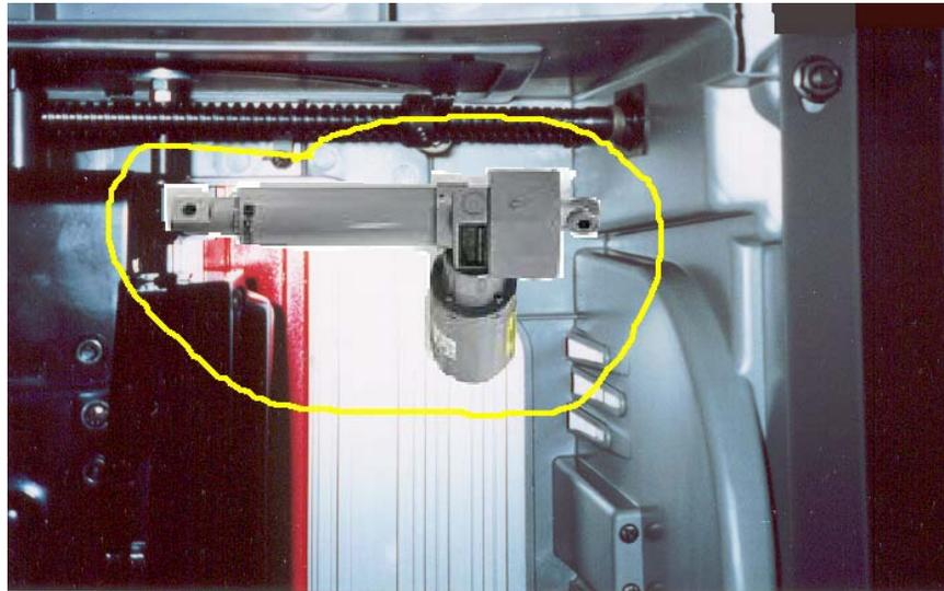
Figure 12. Linear Actuator Angle Adjustment Concept
