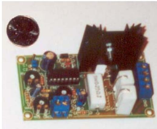
Figure 6. DC to Pulse Width Modulator
