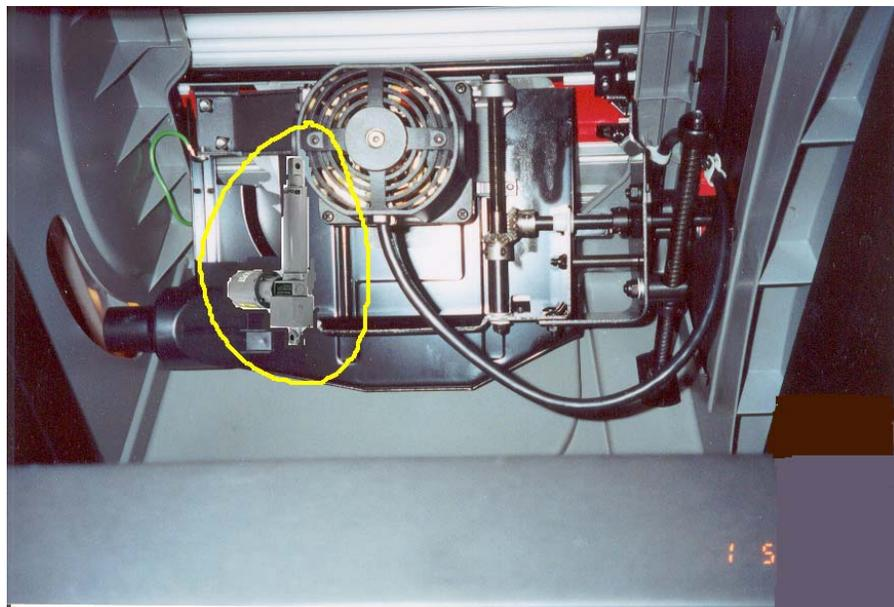
Figure 13. Linear Actuator Height Adjustment Concept
