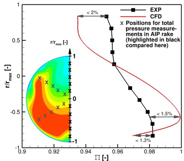
Figure 6. Vertical total pressure profile within the AIP of duct 2 at MPS in the SETF
