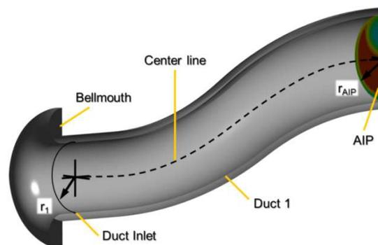
**Figure 3. Duct geometry 1 (generic inlet duct)**
