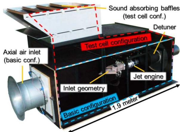
**Figure 2. Scaled Engine Test Facility (SETF)**
