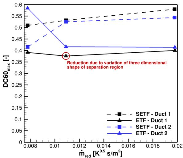
Figure 10. Total pressure distortions
