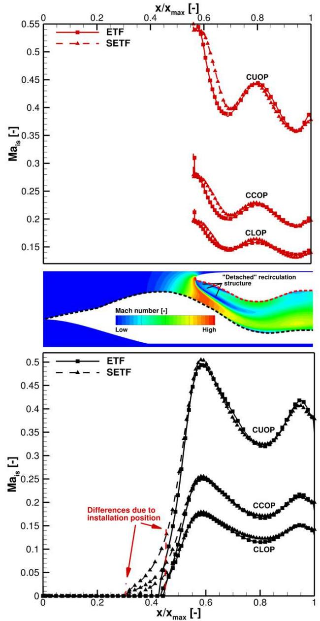
Figure 9. Isentropic Mach numbers on the symmetry plane surface of duct geometry 2 for three corresponding engine operating points
