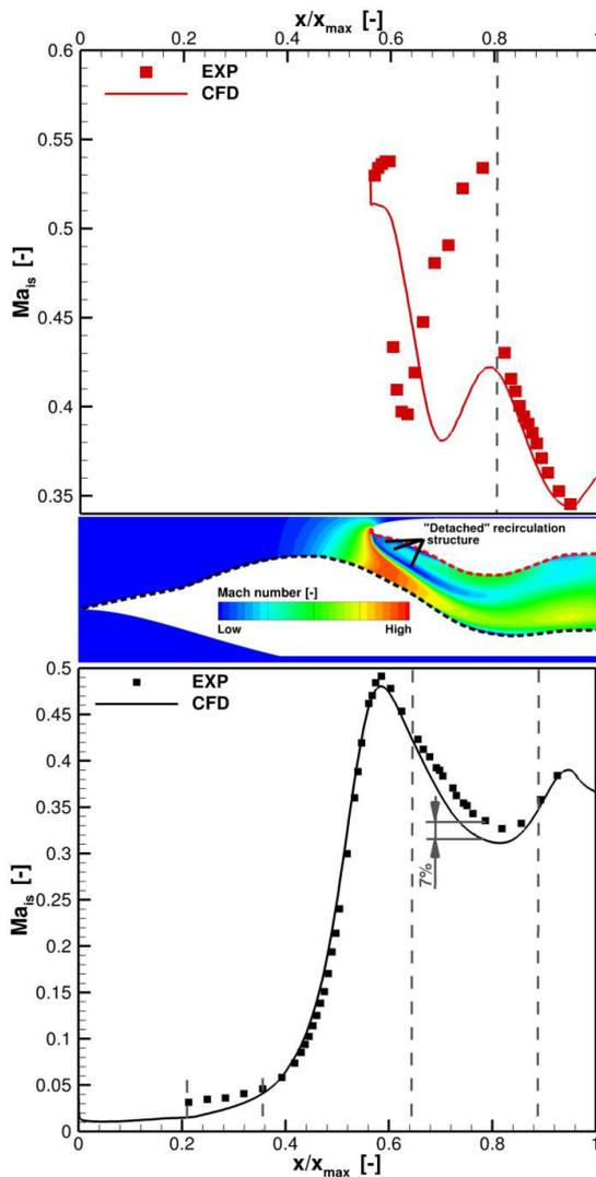
Figure 5. Isentropic Mach number on the symmetry plane surface of duct geometry 2 at MPS in the SETF (test cell configuration)
