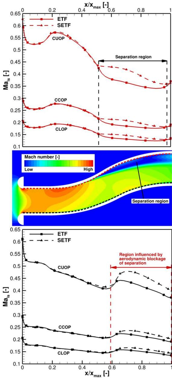
Figure 8. Isentropic Mach numbers on the symmetry plane surface of duct geometry 1 for three corresponding engine operating points
