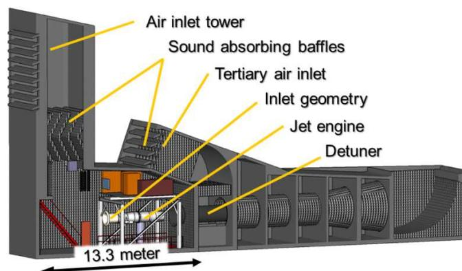
**Figure 1. Engine Test Facility (ETF)**
