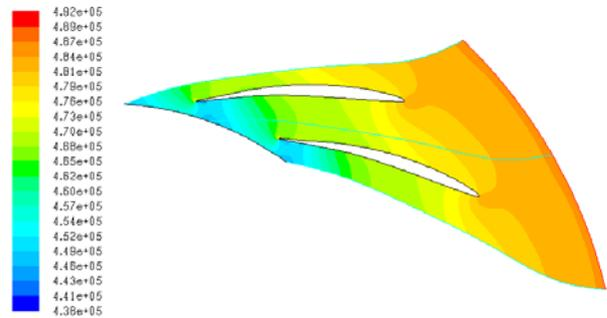
**Fig. 10** Static Pressure Contour of Diffuser Cascade
