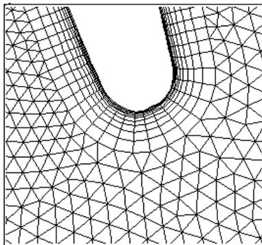
**Fig. 4** Mesh near trailing edge
