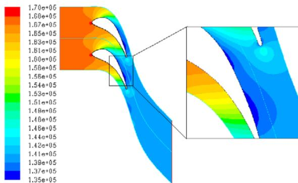
**Fig. 5** Static Pressure Contour of Turbine Cascade
