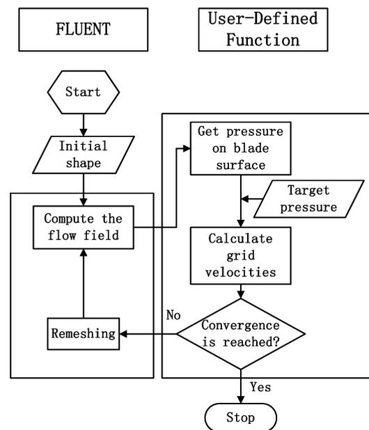
**Fig. 2** Flow Chart of Inverse Design Method
