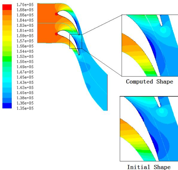
**Fig. 9** Static Pressure Comparison of Turbine Cascade
