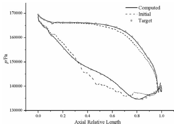
**Fig. 7** Pressure Distribution Comparison of Turbine Cascade
