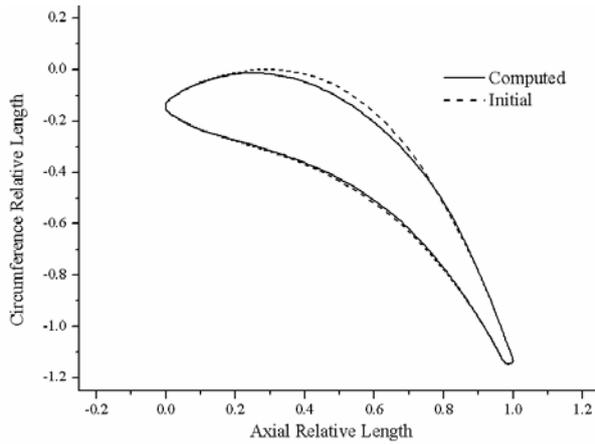
**Fig. 8** Shape Comparison of Turbine Cascade
