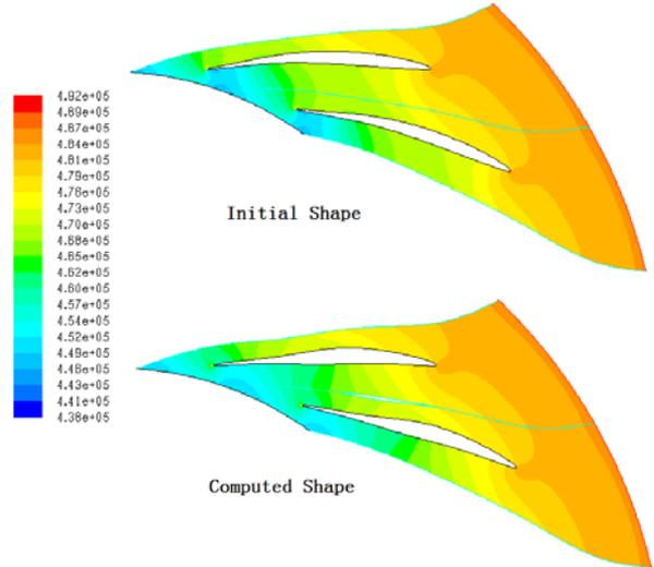
**Fig. 14** Flow Field Comparison of Diffuser Cascade
