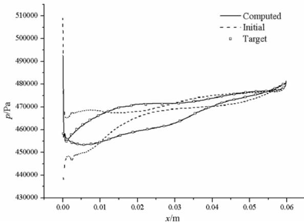
**Fig. 12** Pressure Distribution Comparison of Diffuser Cascade
