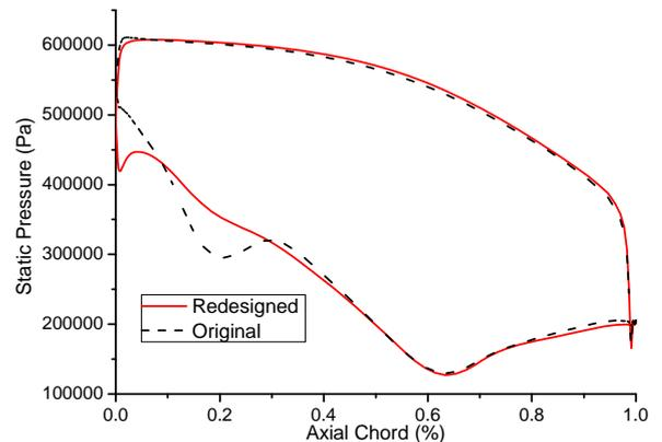
Fig. 6. Static pressure distribution on the blade surfaces at 95% span
