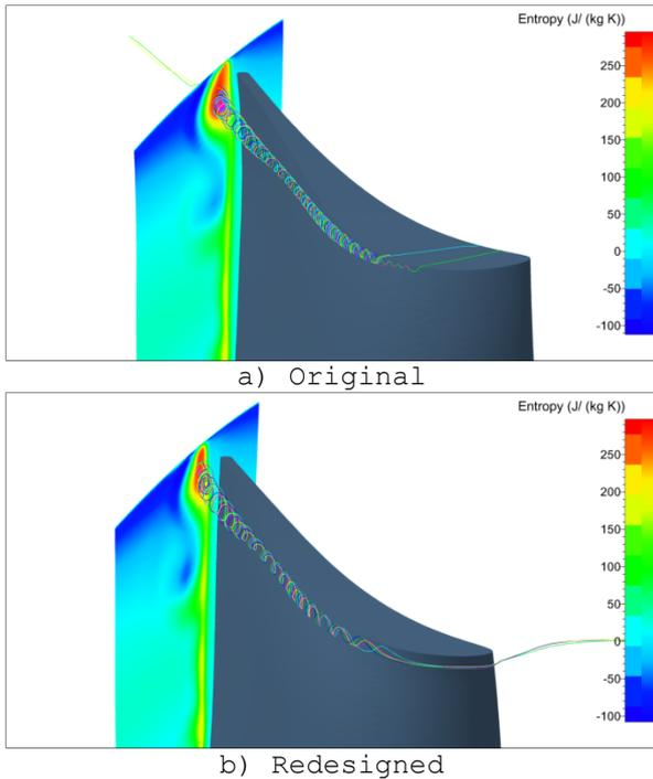
Fig. 5. Streamlines passing through the tip leakage vortex for the original case and redesigned case
