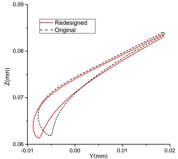
Fig. 1. Blade tip profiles of the original case and redesigned case
