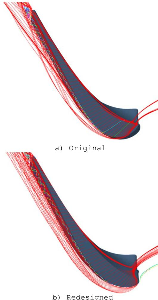
Fig. 7. Projection of the streamlines passing through the blade tip gap for the original case and redesigned case
