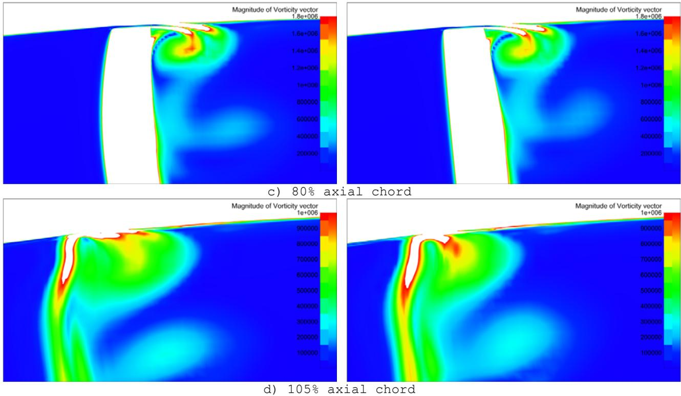
Fig. 8. Vorticity distribution in blade tip region at 25%, 40%, 85% and 105% axial chord
