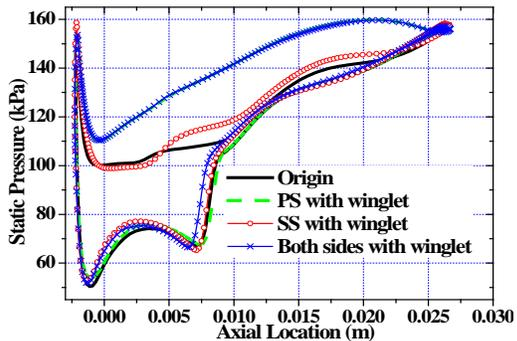
**Fig.14 The static pressure distributions along blade surface edge over tips near stall point of rotors with the same back pressure**
