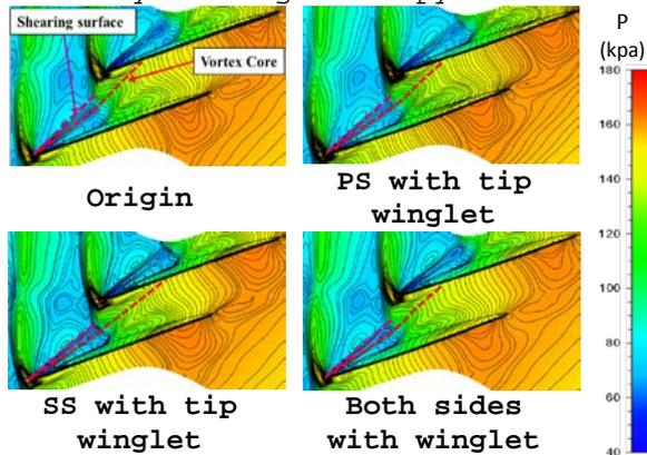
**Fig.12 The contours of static pressure in mid-span of tip gap near stall point of rotor with the same back pressure**
