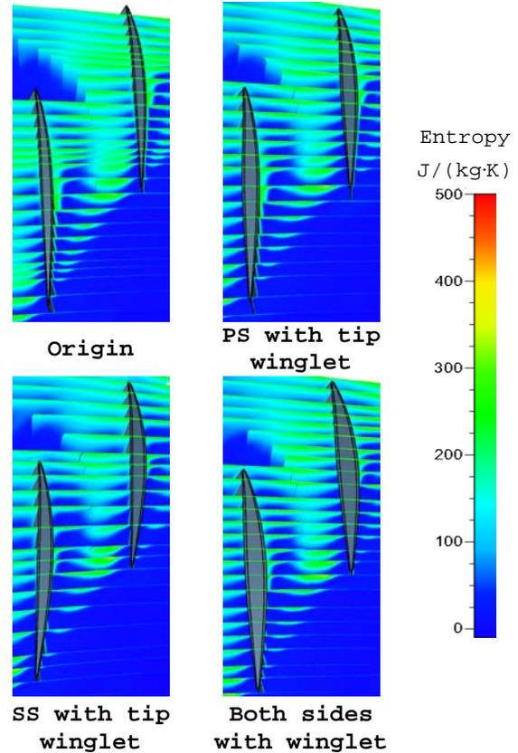
**Fig.18 The distributions of entropy in tip region of rotor near stall point with the same back pressure**
