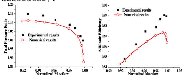
**Fig.4 Overall performance of Rotor 37 at design condition**
