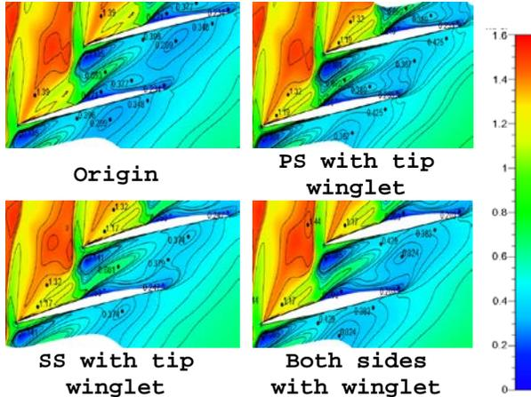
**Fig.17 The contours of relative Mach number in blade tip region near stall point of rotor with the same back pressure**
