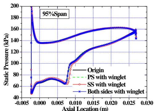
**Fig.19 Distributions of static pressure near surface at different span of rotor near stall point with the same back pressure**
