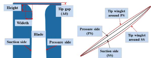
**Fig.1 Structure of tip winglet**
