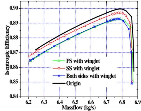
Fig.6 Characteristics of rotors with different location and the same size of tip winglet
