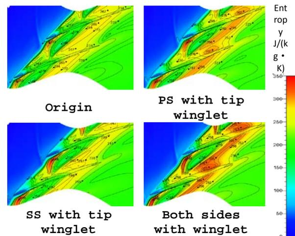
**Fig.13 The contours of entropy at mid-span of tip gap near stall point of rotors with the same back pressure**
