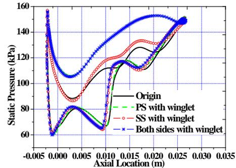
**Fig8. The static pressure distributions along blade surface edge over tips at peak efficiency point of rotors**
