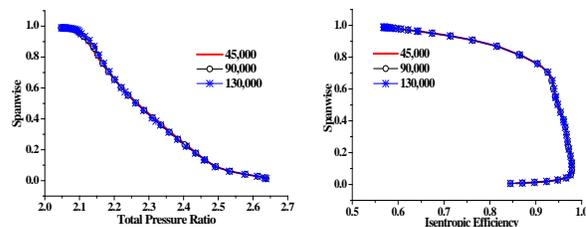
**Fig.3 Spanwise distributions of pressure ratio and efficiency at exit of original rotor**
