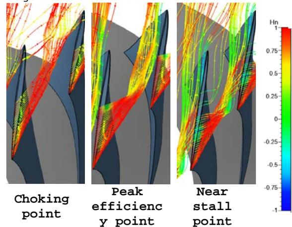
**Fig.9 Distribution of  $Hn$  along streamlines of relative flow in tip region of rotor at different conditions**
