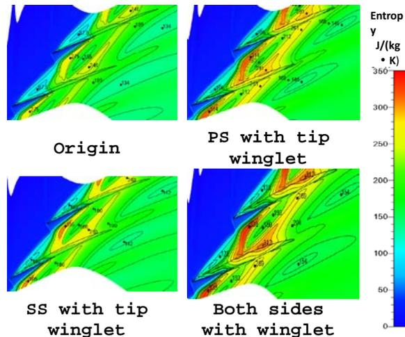
**Fig.7 The contours of entropy at mid-span of tip gap at peak efficiency point of rotors**
