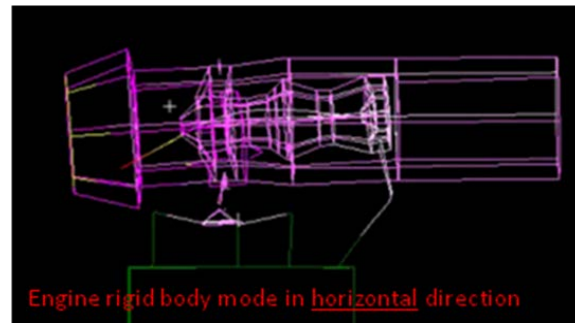
Figure 8: Engine rigid body mode in horizontal direction.
