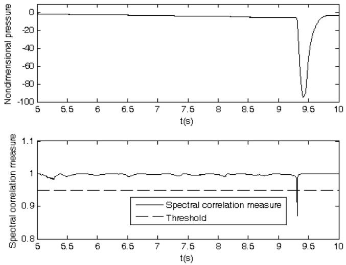
Fig 6. Detecting result of the C2 with total pressure of outlet
