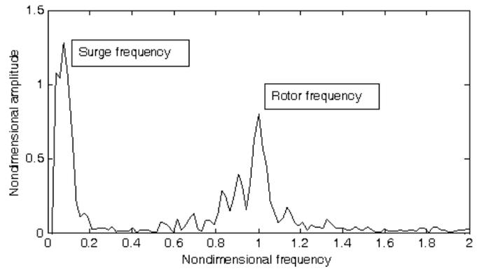
Fig 2. Spectrum of pressure signal in surge state
