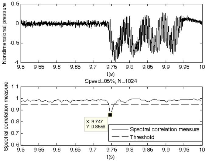
Fig 11. Detecting result of the C1 at 85% speed with N=1024
