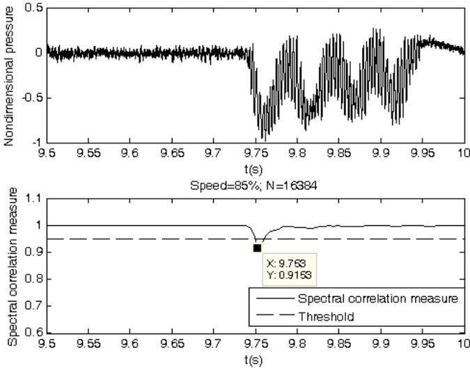
Fig 12. Detecting result of the C1 at 85% speed with N=16384
