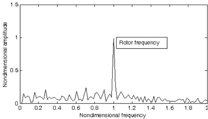
Fig 1. Spectrum of stable pressure signal
