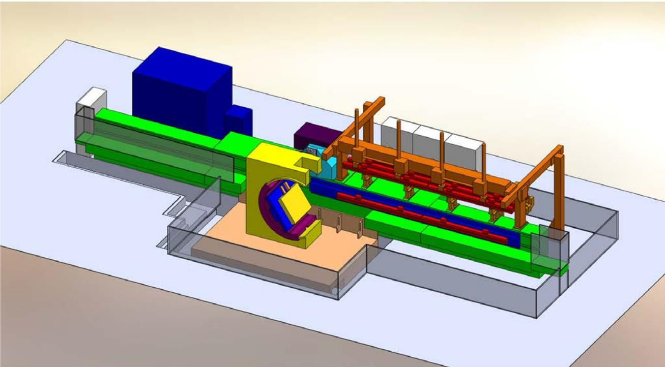
What is often missed when cycle times are calculated is the extensive pre-setting of the 8 to 14 broach-cutter-segments. All of these segments must be positioned and aligned in their Broach-Bar, then torqued down. Many hours are spent in this phase of set-up, just shimming and adjusting each of the segments, only to find a dulling cutter later needs exchanging, repeating the adjusting procedure.
