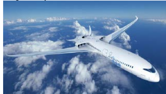
Figure 3 E-Thrust (DEAP) concept aircraft
