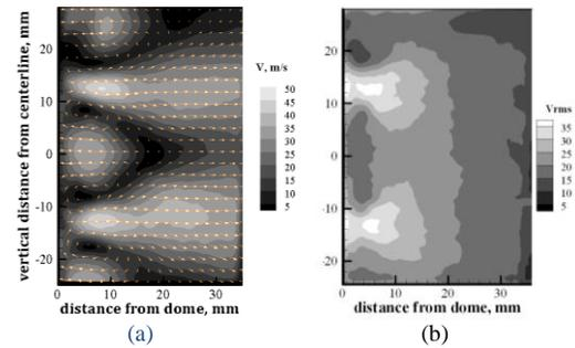
Figure 5. Average velocity field (left) and RMS of velocity (right) within the vertical center plane, computed from 500, 2-D image pairs.  $T_3 = 828K$ ,  $P_3 = 1034\text{-kPa}$ . Flow left to right.
