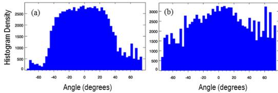
Figure 12. Drop Occurrences at angles relative to center of air mixer exit for liquid through the 7-point LDI center element and no flow to the outer elements.  $T_3=650K$ ,  $P_3=217.1\text{-kPa}$ , air flow rate =  $0.107\text{ kg/s}$ , reference velocity= $9.1\text{ m/s}$ . (a): water flow, at  $7.01\text{ kg/h}$ ; (b): JP-8, at  $5.65\text{ kg/h}$ .
