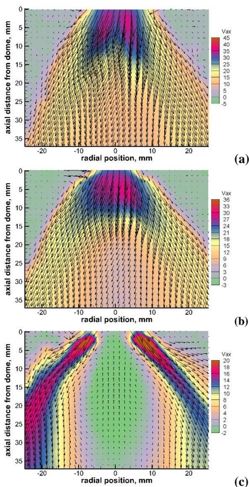
Figure 8. 1-point LDI. PIV average velocity fields in center plane for water spray with injector tip at the venturi throat.  $T_3 = 700K$ ,  $P_3=217.1-kPa$ , air flow rate =  $0.107 kg/s$ , reference velocity=  $9.1 m/s$ , water flow rate=  $3.89 kg/h$ . Increasing air swirler angle from left to right: (a) 45 degrees, (b) 52.5 degrees, (c) 60 degrees. The flow is from top to bottom.
