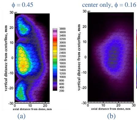
Figure 6. On-chip integrated averages of  $CH^*$  at  $T_3 = 617K$ . Left:  $\phi = 0.45$ , evenly fueled. Right: center-only fueled, with  $\phi_{local} = 1.45$  and  $\phi_{total} = 0.16$ . Flow is left to right.
