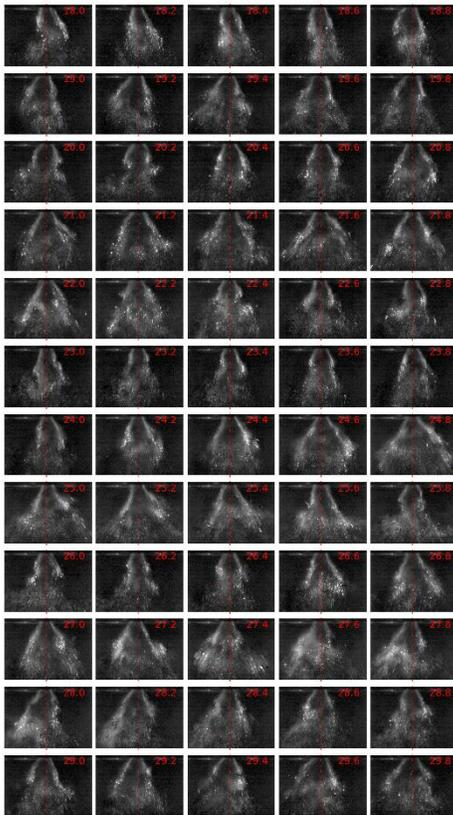
Figure 13. Individual movie frames from center-only "fueling" using water in the 7-point LDI.  $T_3 = 650K$ ,  $P_3=217.1\text{-kPa}$ , air flow rate =  $0.107\text{ kg/s}$ , reference velocity =  $9.1\text{ m/s}$ , water flow rate =  $3.89\text{ kg/h}$ . Flow from top to bottom.
