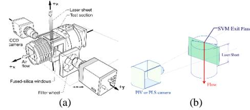
Figure 4. Illustrations showing flame tube shape, general orientation, and window access used for typical 2-D imaging experiments: a) 9-point LDI, with laser sheet passing through the flow vertically; b) 1-point and 7-point LDI, with laser sheet travel horizontal tests.
