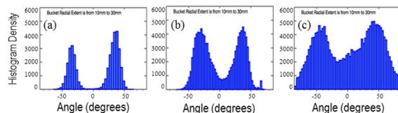
Figure 9. Occurrences of droplets at angles relative to center of air mixer exit with injector tip at the venturi throat.  $T_3 = 700K$ ,  $P_3=217.1-kPa$ , air flow rate =  $0.107 kg/s$ , reference velocity=  $9.1 m/s$ , water flow rate=  $3.89 kg/h$ . Air swirler: (a)  $45^\circ$ , (b)  $52.5^\circ$ , (c)  $60^\circ$ .
