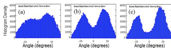
Figure 10. Occurrences of droplets at angles relative to center of air mixer exit with injector tip at the venturi throat.  $T_3 = 700K$ ,  $P_3=217.1-kPa$ , air flow rate =  $0.143 kg/s$ , reference velocity=  $12.2 m/s$ , water flow rate=  $4.09 kg/h$ . Injector tip distance upstream of the throat in throat diameters: (a) 0, (b) 0.16, (c) 0.31
