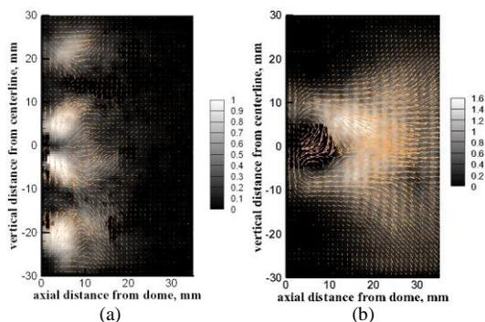
Figure 7. Average Flame/Flow structure derived using PIV-type processing of 9000 consecutive high-speed image pairs.  $T_3 = 828K$ . Left: Nine injectors fueled equally. Right: Center injector fueled only.
