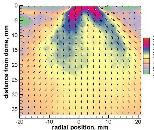
Figure 11. 7-point LDI: Average PIV velocity fields at vertical center plane for water spray, liquid from center nozzle only.  $T_3 = 650K$ ,  $P_3=217.1-kPa$ , air flow rate =  $0.107 kg/s$ , reference velocity=  $9.1 m/s$ , water flow rate=  $3.89 kg/h$ . The flow is from top to bottom.
