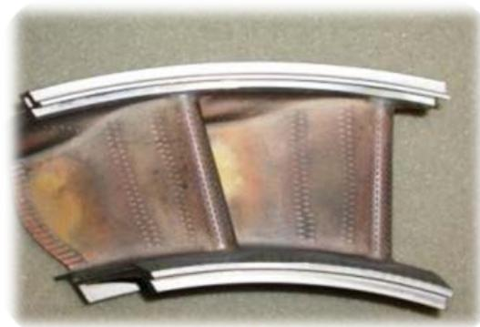
**Figure 2.** Turbine vanes with cooling holes
