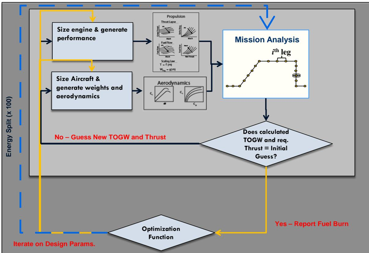
Figure 2: Traditional MDAO Process Applied to Adaptive Technology
