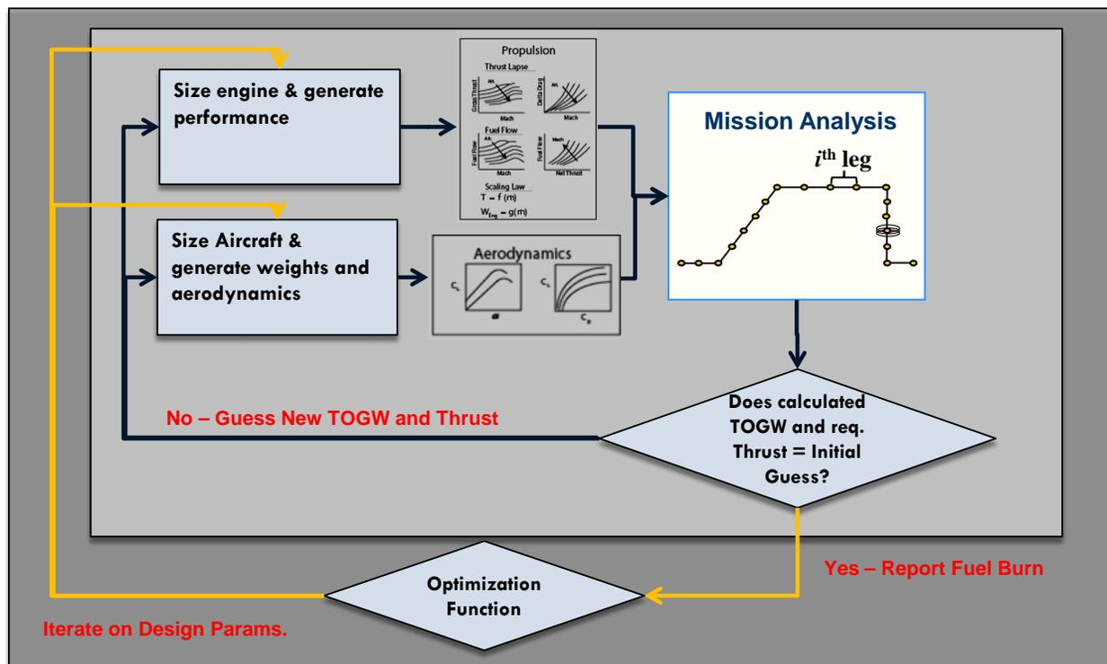
Figure 1: Traditional MDAO Process (Optimizer External to Analysis)
